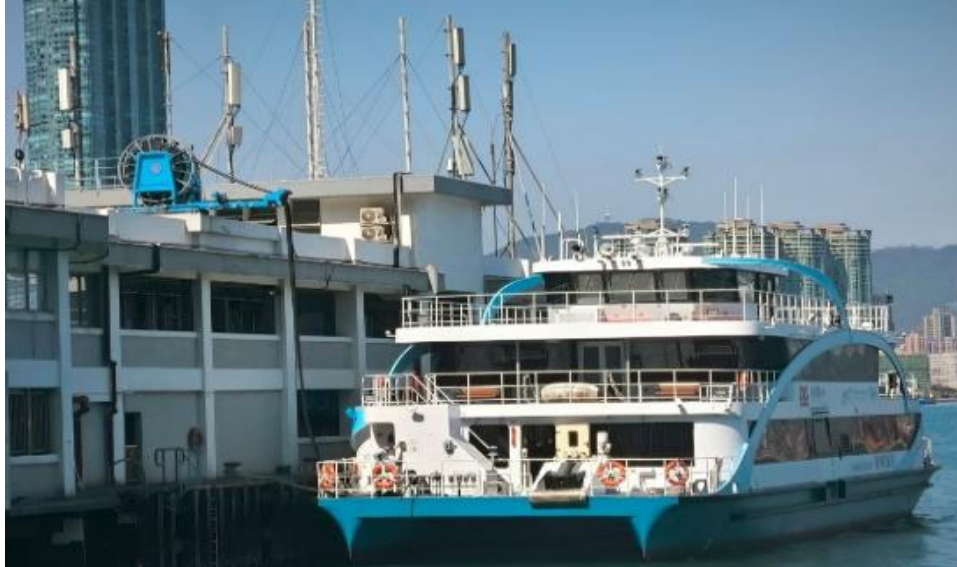
Hong Kong's pioneering electric ferry, the "Xin Ming Zhu XXXIX", docked alongside its shore charging equipment.
