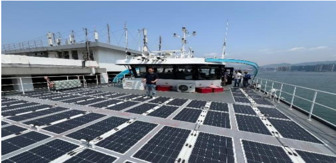
Members inspected the navigation bridge and solar panel layout on the upper deck.
